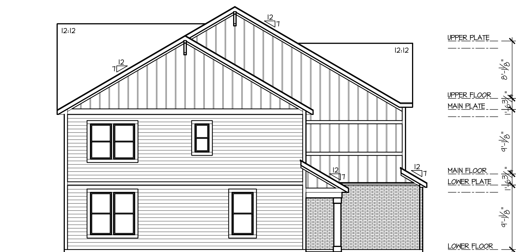
Building Type A - Left End Condition
