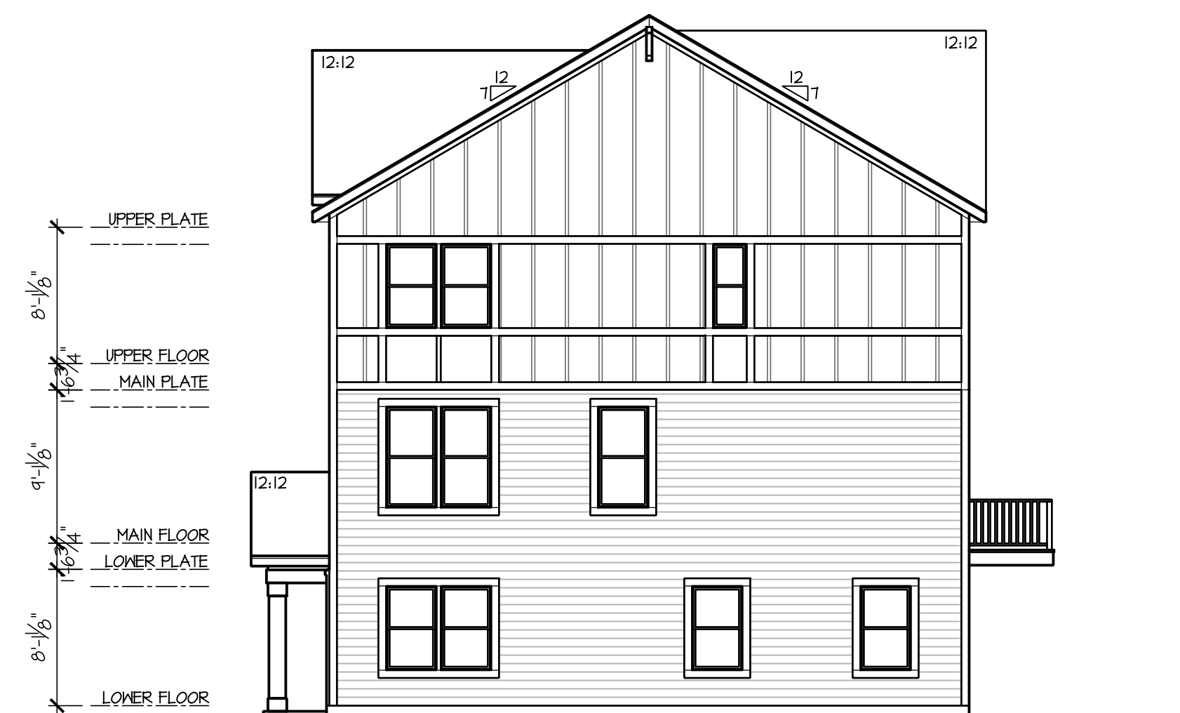
Building Type B - Right End Condition
