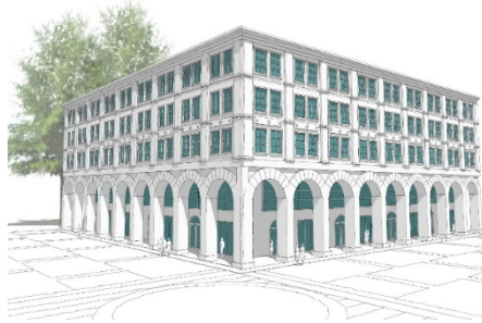
FIGURE 20.36-19: ARCADE/STRUCTURAL CANOPY FRONTAGE
