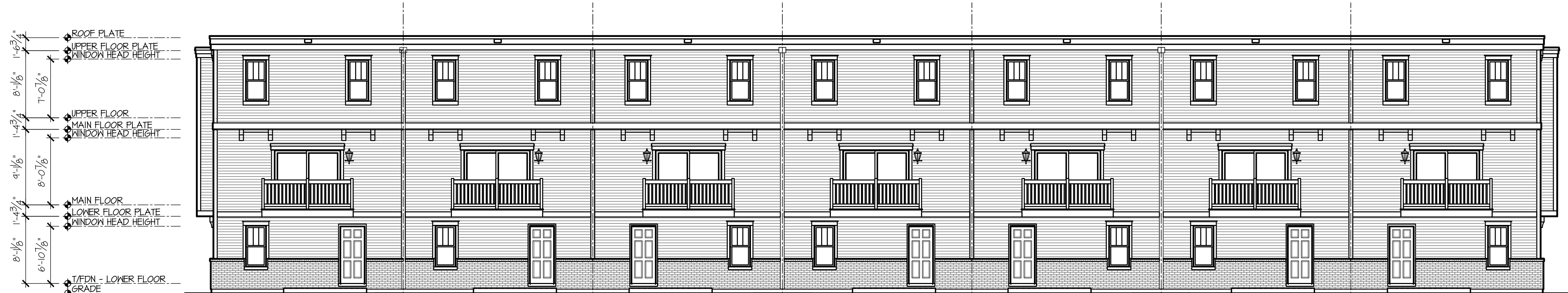
7-Unit Building Rear Elevation SCALE: 1/8"=1'-0"
