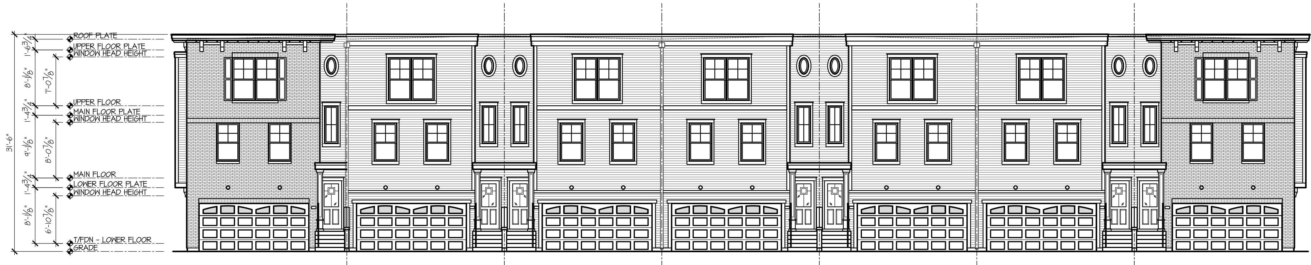
7-Unit Building Front Elevation SCALE: 1/8"=1'-0"
