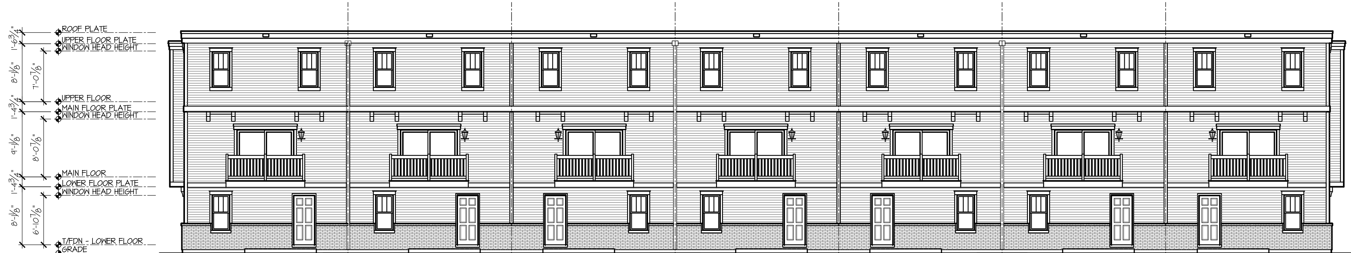
7-Unit Building Rear Elevation SCALE: 1/8"=1'-0"
